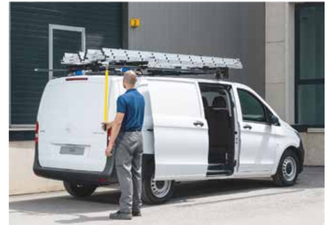
5. The Auto Clamp secures the ladder without additional straps or clamps.
