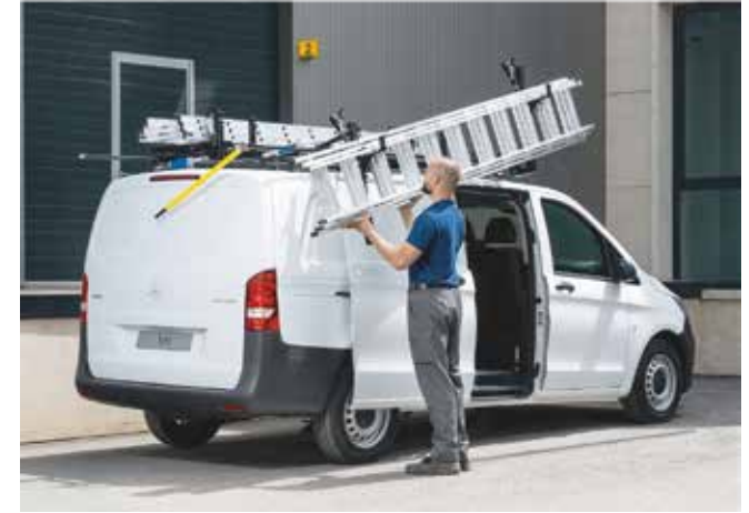
2. Lift the rear end of the ladder on to the rear hook.
