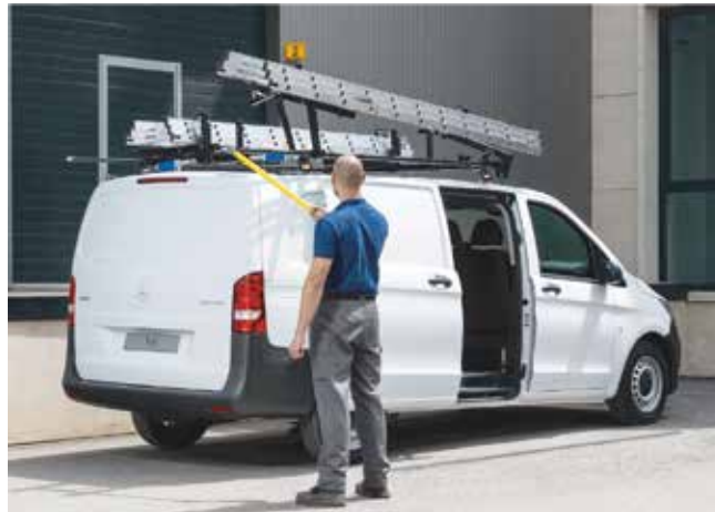
4. Pull the handle to rotate the ladder onto the roof walking backwards with your arm straight
