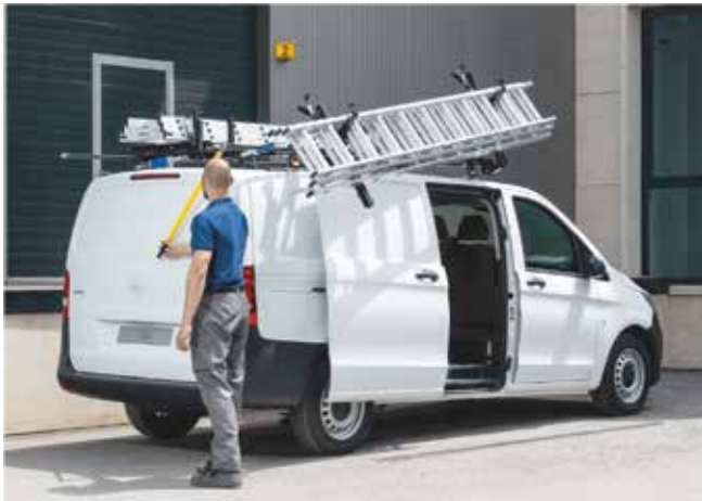
3. For high roof vehicles: lift the slide upwards until it is locked position.
