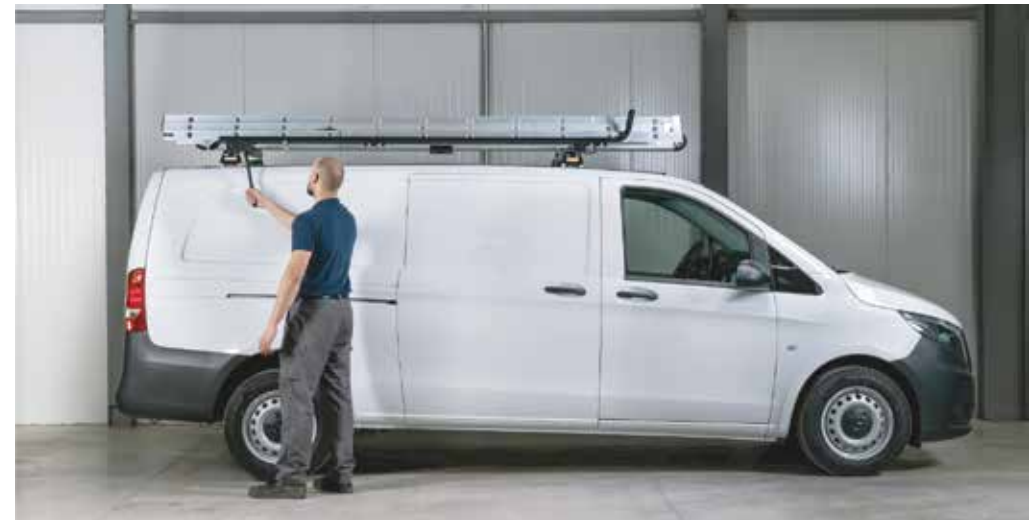
3. Turn the handle to swing the hook upward and clamp the ladder tightly into place
